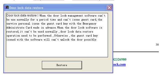
When the door lock management software can't be use normally for a period time and can't issue guest card ,the service personal issue the guest card key with the Emergency Administrate Card made in advance.When the door lock software is restored ,it can't be used normally ,door lock data restore operation need to be performed ,Otherwise ,the guest card key issued with the software will can't unlock the door possibly.
